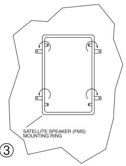
STEP 3: Insert Ring into the Sheetrock & Bend Mounting Tabs around behind the Sheetrock
